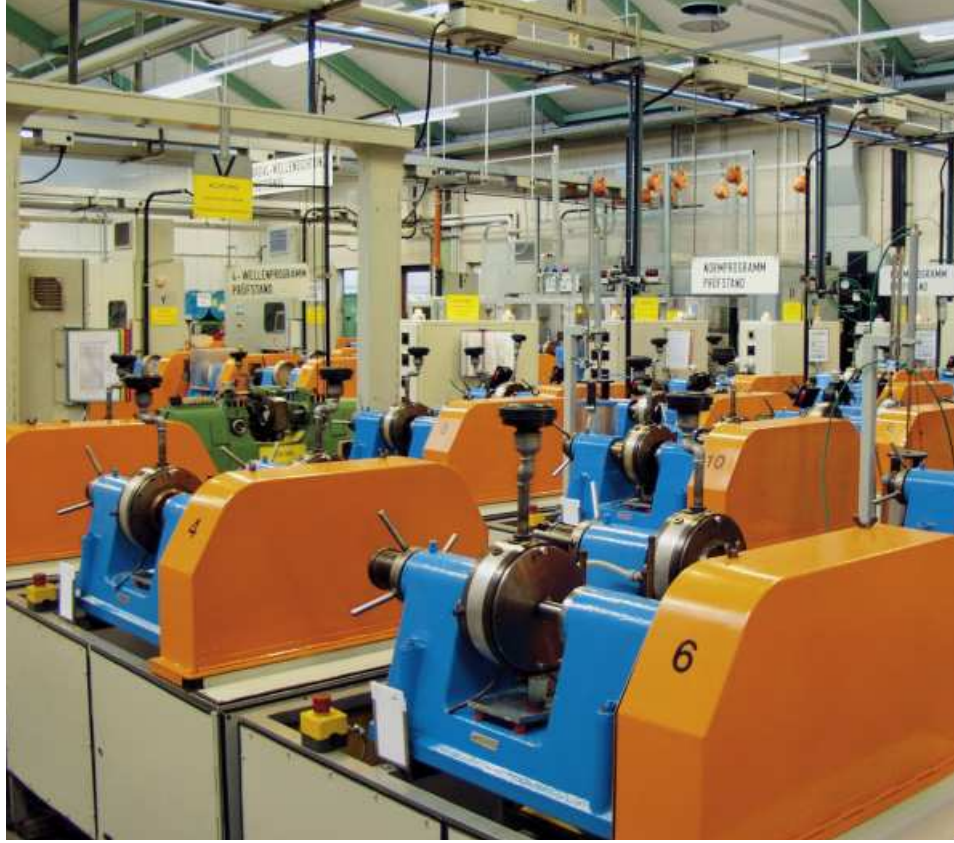
The Simmerring test fields at Simrit are equipped with many special installations, in addition to standard test benches.
